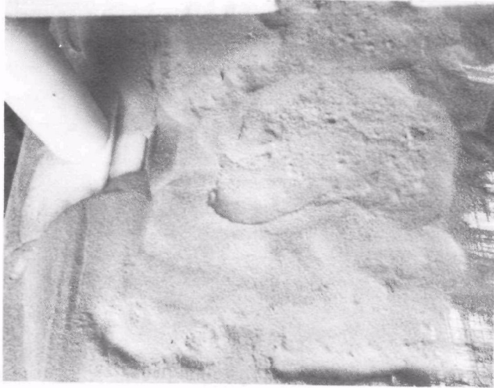
Blown dust layer, large particles > 25 \mu\text{m} (Temp 86°C, Moisture 12 V /O)
