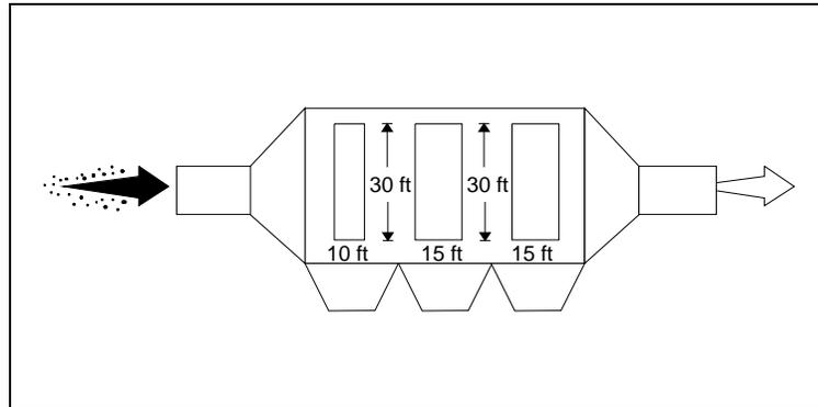
An ESP with the above configuration has the following aspect ratio:
